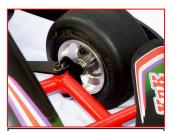
Heavy duty Knuckle with 20mm Stub Axles - replaceable.
